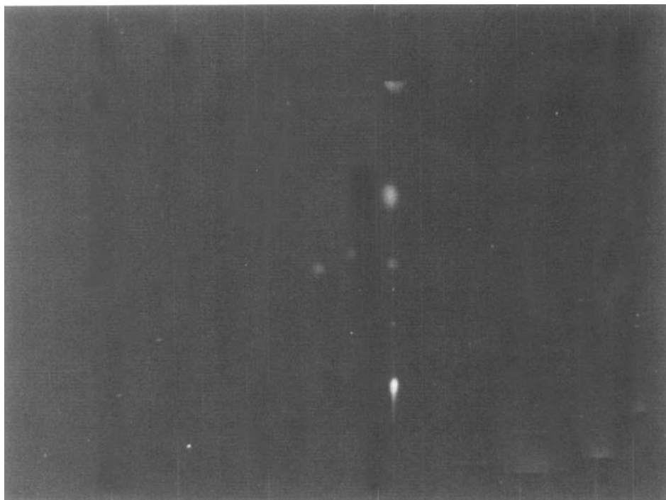
Fig.12. TLC separation of MK0912 using \gamma -cyclodextrin in the spotting solvent and HDTAB in the mobile phase. Left channel: MK0912; right channel: crude sample. For chromatographic conditions see text
